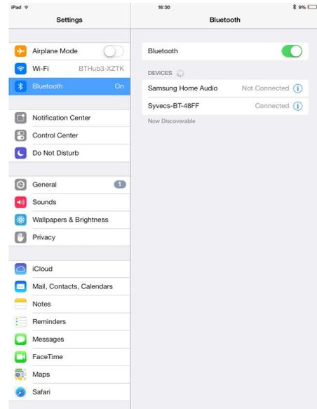
The mobile device will then find the Syvecs Bluetooth Module which will appear as "Syvecs-BT – XXXX" XXXX is the Serial number of the device.... Connect to the unit
