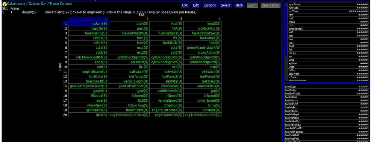
In the unlikely event that the Gauges are displaying the wrong values on the App. Head to the Custom Stream Config under the Settings tab. Here you are able to change the Stream Config to match your Syvecs output stream.
