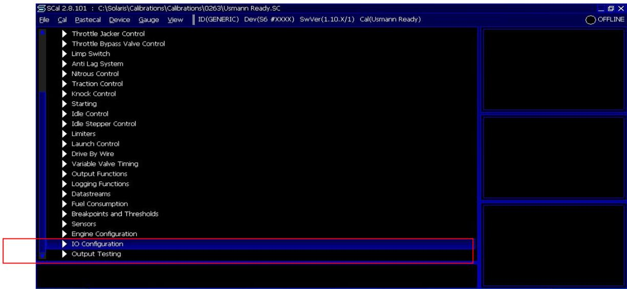
After selecting **IO Configuration**, Select **Pin Assignments** the Full Input and output table will be brought up.
